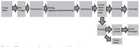
Fig. 1. The processing of cocoa beans (own elaboration)
